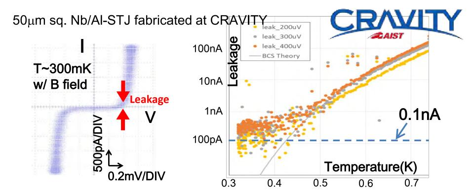
$I_{leak}$ ~200pA for 50µm sq. STJ, and achieved 50pA for 20µm sq. This satisfies our requirement!
