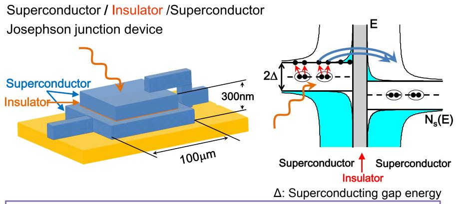
A constant bias voltage ( $|V| < 2\Delta$ ) is applied across the junction. A photon absorbed in the superconductor breaks Cooper pairs and creates tunneling current of quasi-particles proportional to the deposited photon energy.
