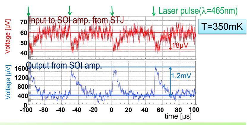
Demonstrated to show amplification of Nb/AI-STJ response to laser pulse by SOI amplifier situated close to STJ at T=350mK
