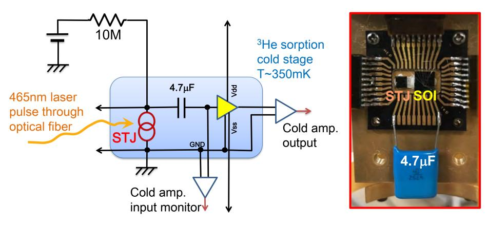
We connect 20 $\mu m$  sq. Nb/Al-STJ and SOI amplifier on the cold stage through a capacitance
