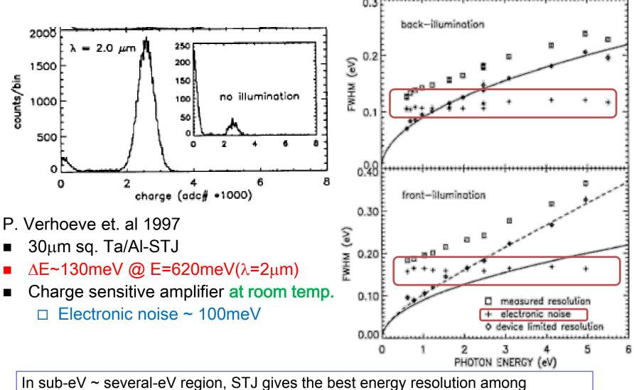
superconductor based detectors, but limited by readout electronic noise.
