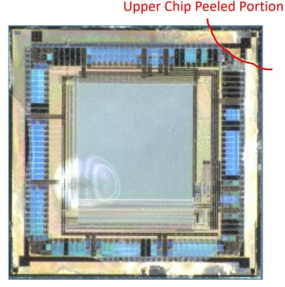
Proton irradiation : 400 kGy ( $5 \times 10^{14}$  cm<sup>-2</sup> in 1 MeV neutron equivalent)
