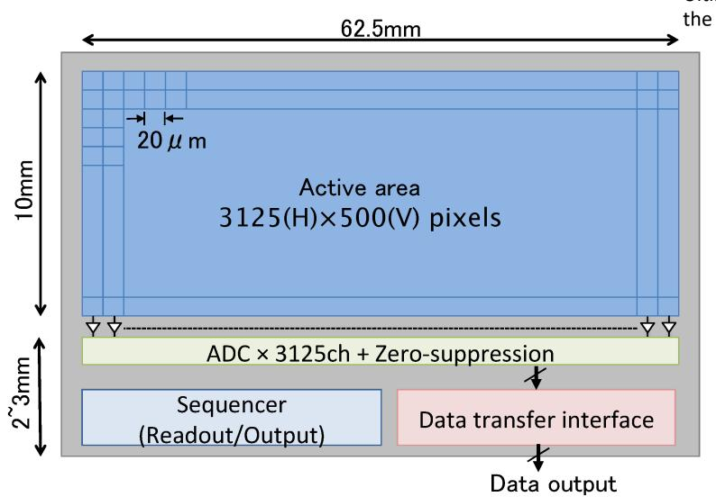
Ultimate layout to fit in the ILD vertex geometry
