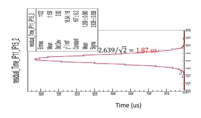
Time resolution <2us is demonstrated from test beam data
