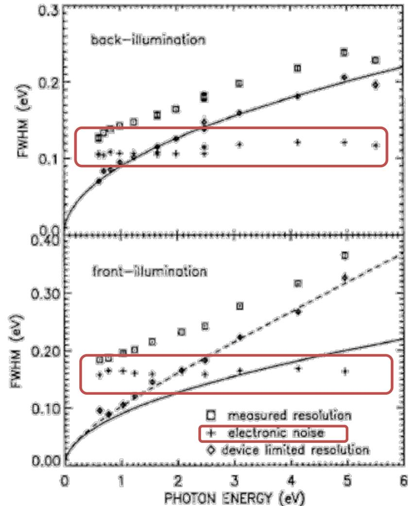
In sub-eV  $\sim$  several-eV region, STJ gives the best energy resolution among superconductor based detectors, **but limited by readout electronic noise.**
