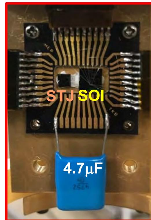
We connect 20 $\mu\text{m}$  sq. Nb/Al-STJ and SOI amplifier on the cold stage through a capacitance
