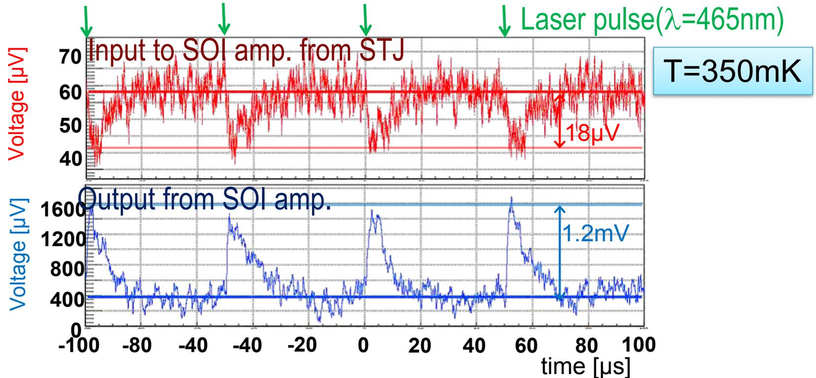
Demonstrated to show amplification of Nb/Al-STJ response to laser pulse by SOI amplifier situated close to STJ at  $T = 350 \text{ mK}$
