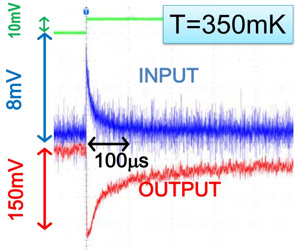
Test pulse input through  $C=1\text{nF}$  at  $T=3\text{K}$  and  $350\text{mK}$
