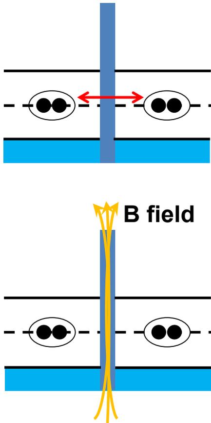
Tunnel current of Cooper pairs (Josephson current) is suppressed by applying magnetic field
