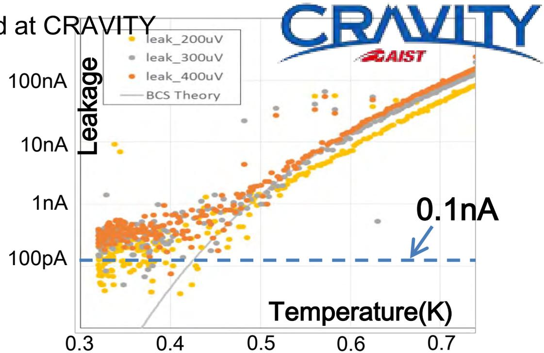
$I_{\text{leak}} \sim 200\text{pA}$  for 50 $\mu\text{m}$  sq. STJ, and **achieved 50pA for 20 $\mu\text{m}$  sq.**
