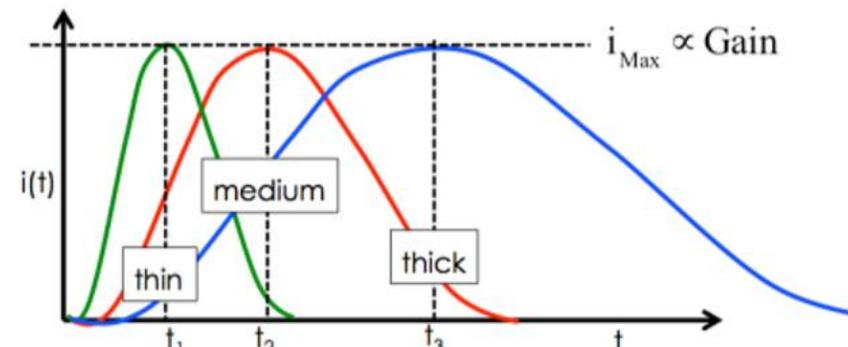
Thicker active sensor will not improve pulse amplitude, degrading the rise time
