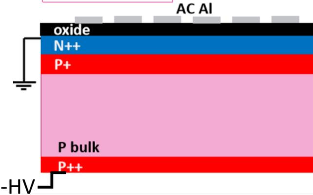
Signals are read out via AC coupled electrodes
