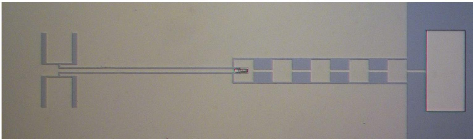
An antenna-coupled Nb-SIS photon detector
