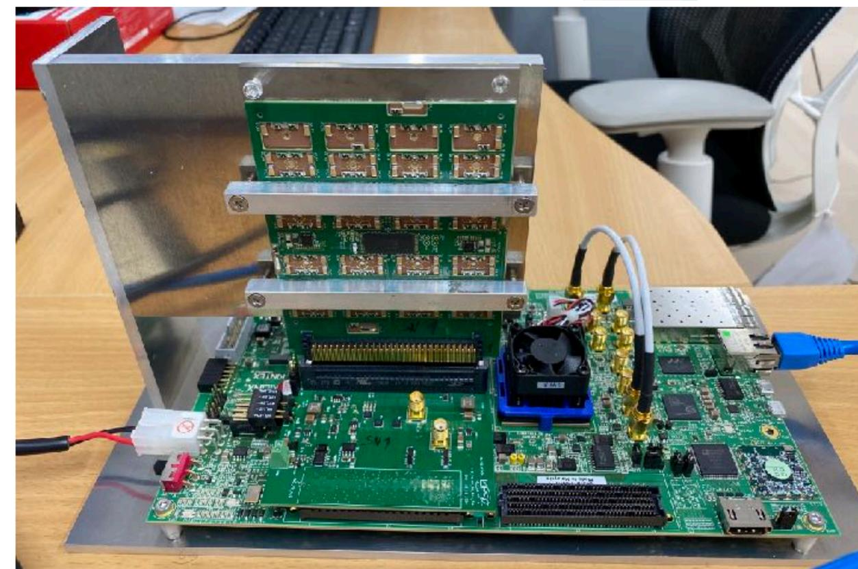
TEST module of FoCal-E pad with HGCROC
