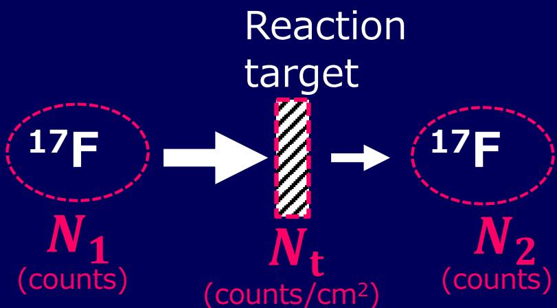
For counting  $N_1$  and  $N_2$ , particle identifications both upstream and downstream of the reaction target are needed in the experiment.
