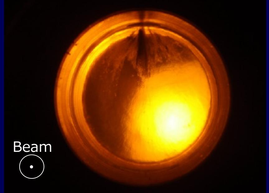
A thick and large SHT (Maximum volume :  $\phi 50 \times 100 \text{ mm}^3$ ) without any void or porous region was developed by optimization of the supply pressure.
